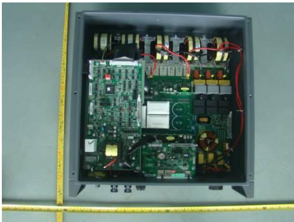
Internal view for EVVO 3000TL3P, EVVO 4000TL3P, EVVO 4800TL3P , EVVO 5000TL3P, EVVO 6000TL3P
