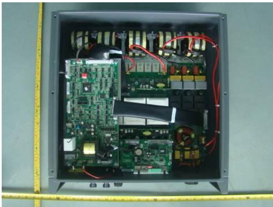
Internal view for EVVO 12000TL3P、EVVO 10000TL3P、EVVO 8000TL3P
